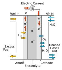
The electrode reactions involved in the working of the H<sub>2</sub>-O<sub>2</sub> fuel cell are as:
